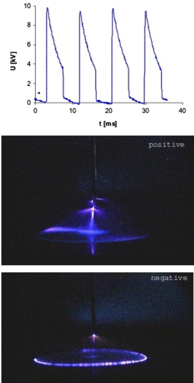
**Fig. 4.** The oscilloscopic record of applied pulsed HV voltage waveform ( $U = 10$  kV,  $f = 100$  Hz) and the corresponding images of the discharges generated in positive and negative polarity above plastic surfaces contaminated with spores.
