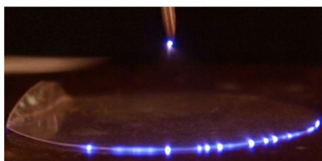
**Fig. 3.** The oscilloscopic record of the current of negative Trichel pulses ( $U = 7$  kV,  $f = 550$  kHz,  $I_{\max} = 0.2$  mA) and the related discharge photo.
