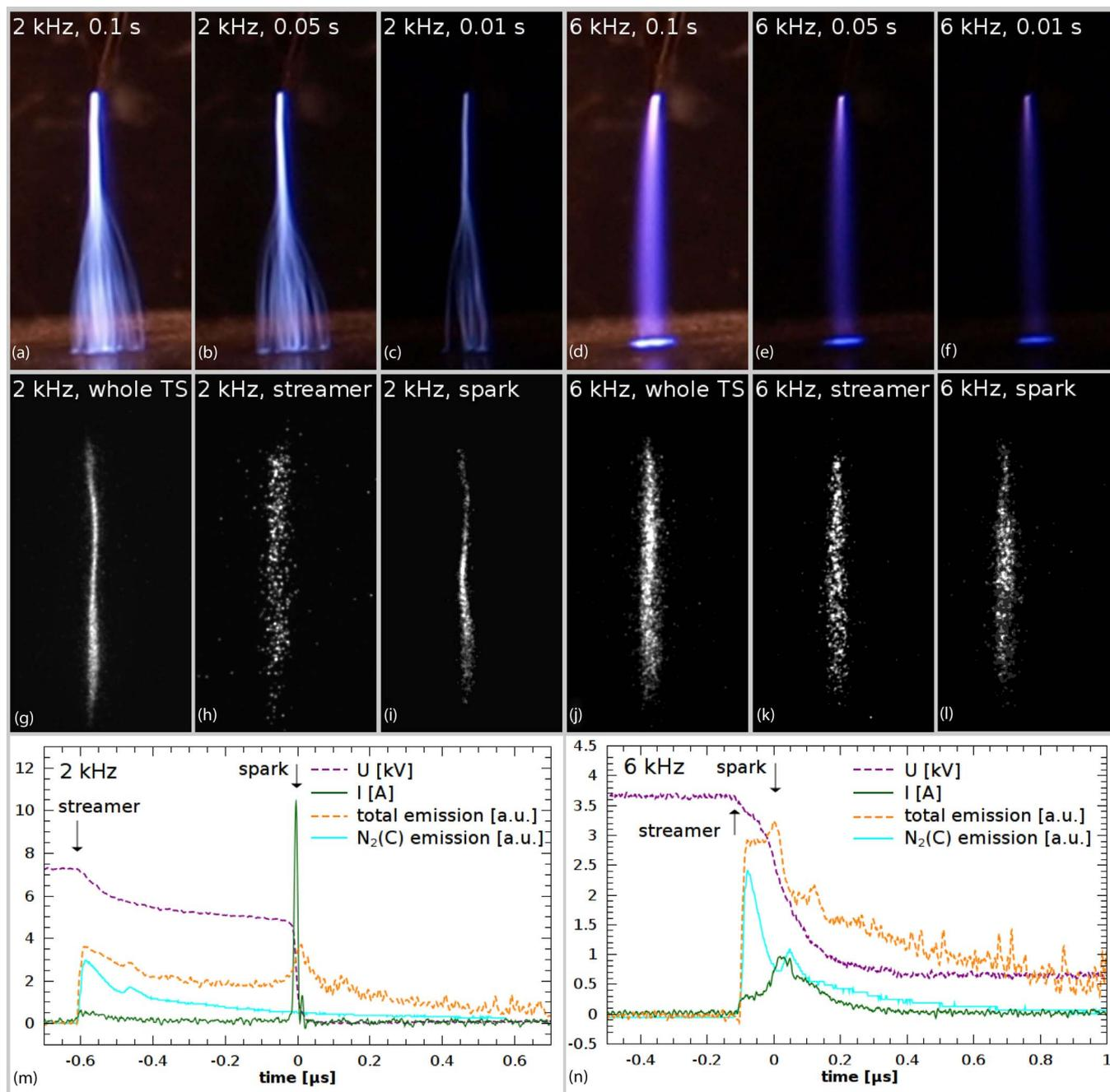
Fig. 1. (a)–(f) Photographic images of TS at 2 and 6 kHz with different exposure times, (g and j—whole TS; h and k—streamer phase; and i and l—spark phase) iCCD images of a single TS channel, and (m and n) typical voltage and current waveforms with PMT signals of the total emission (200–800 nm) and N<sub>2</sub> second positive system at 337 nm.
