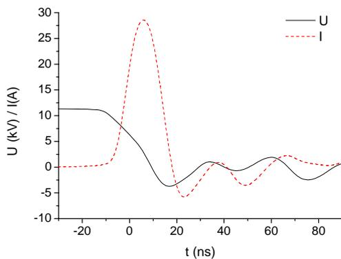
Fig. 3. Typical voltage and current waveforms of TS discharge with electro-spray of water in ns time scale, 10 mm gap.
