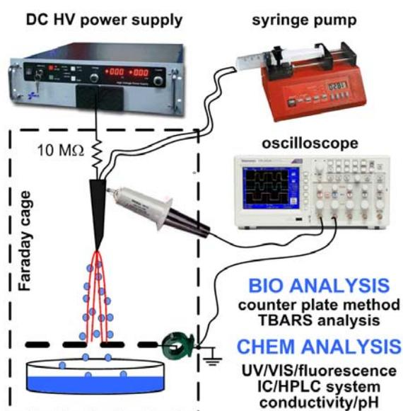
Fig. 1. The experimental setup enabling the contaminated water to be sprayed through the high voltage hollow needle electrode
