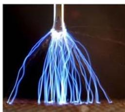
Fig. 2. Photographs of the transient spark with electro-spray of water in 8 mm gap, water flow rate 0.5 mL/min, 9 kV.
