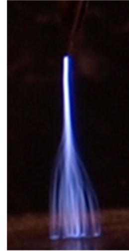
**Figure 3.** Photograph of TS in positive needle-plane gap of 4 mm,  $f = 2 \text{ kHz}$ ,  $R = 6.6 \text{ M}\Omega$  and exposure 0.05 s.
